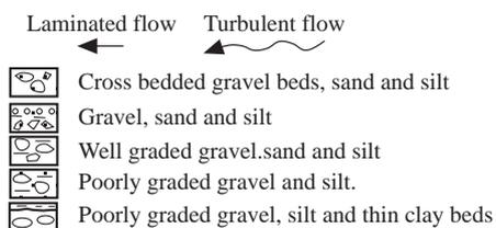
Fine material is washed out along the flow path in places where the flow changes from laminated to turbulent and a hollow is formed. Resettlement of the gravel, and continued washing out of collapsed material, destabilizes the roof of the hollow causing further collapse. The process continues in an upward direction forming a pipe. As the pipe approaches the surface sudden collapse occurs forming a funnel shaped hole (Fig. 7).
